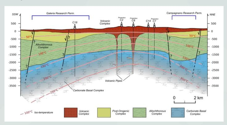
Interpreted N-S cross section of the geological model showing the deep reservoir (Carbonate Basal Complex) and volcanic pipes [Source: STEAM 2023]
